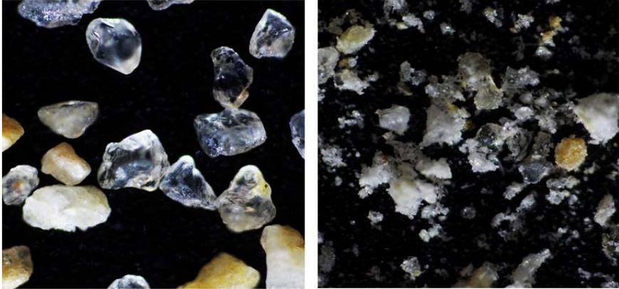
Figure 2 Microscope photos before and after grain crushing
