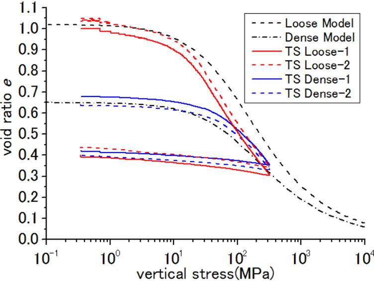
Figure 1 e-log p curve and a fitted M-W model
